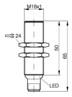
Inductive Sensors BES M18MI-POC50B-S04K M18x1 x 65 normally-closed Sn=5mm shielded
